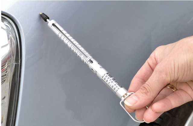
Thickness measurement on automobile paint coating (application example)
