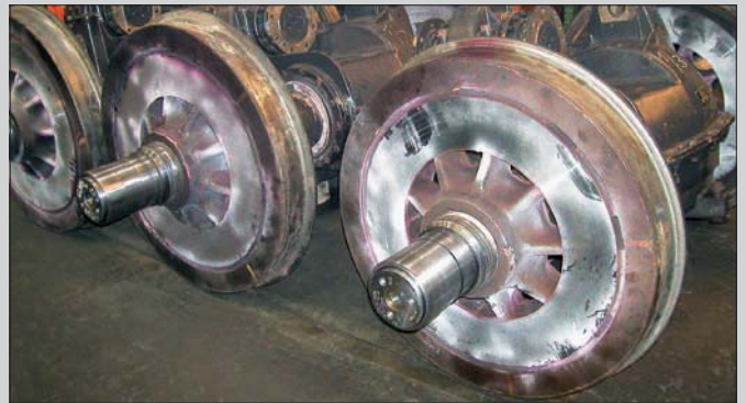
KD-Check penetration testing on railway wheels
