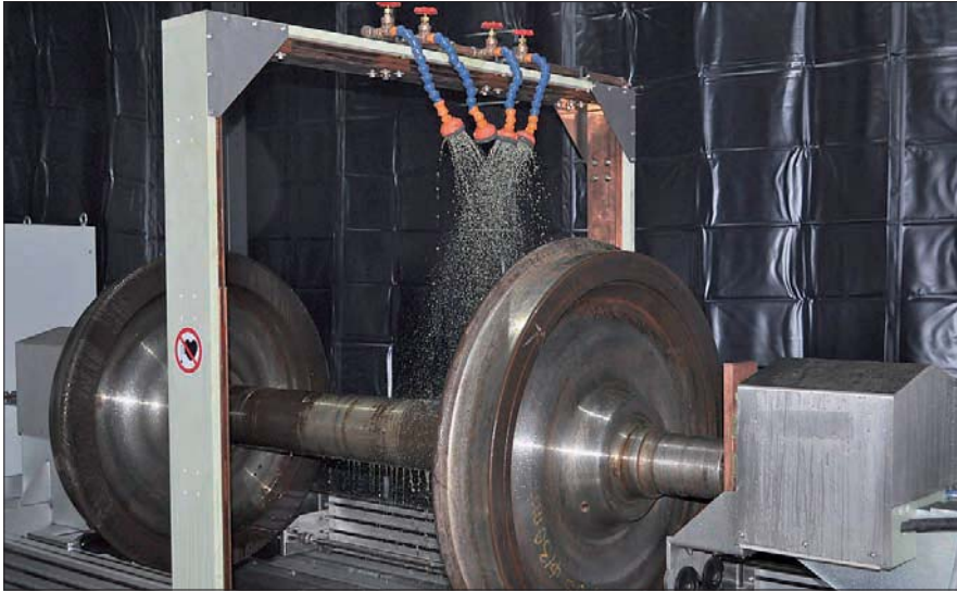
Inspection of railway axle with mounted wheels
