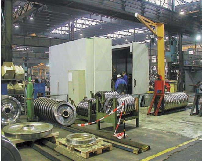
Darkening cabin and crane for loading / unloading.
