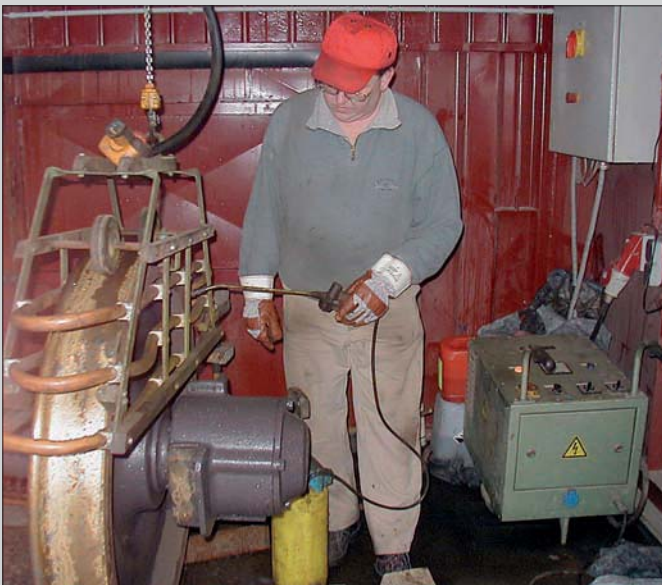
Wheel testing with current flow unit and special high-current coil
