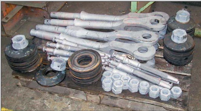
Typical railway components for surface crack detection
