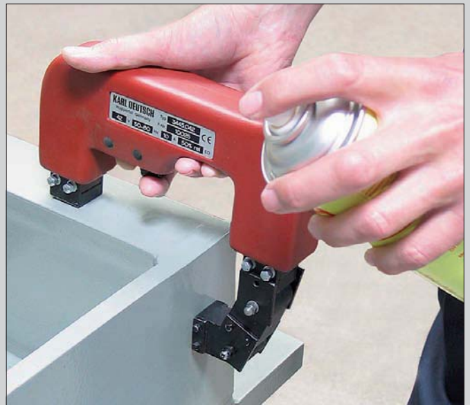
Weld seam testing with DEUTROPULS Hand Yoke.
