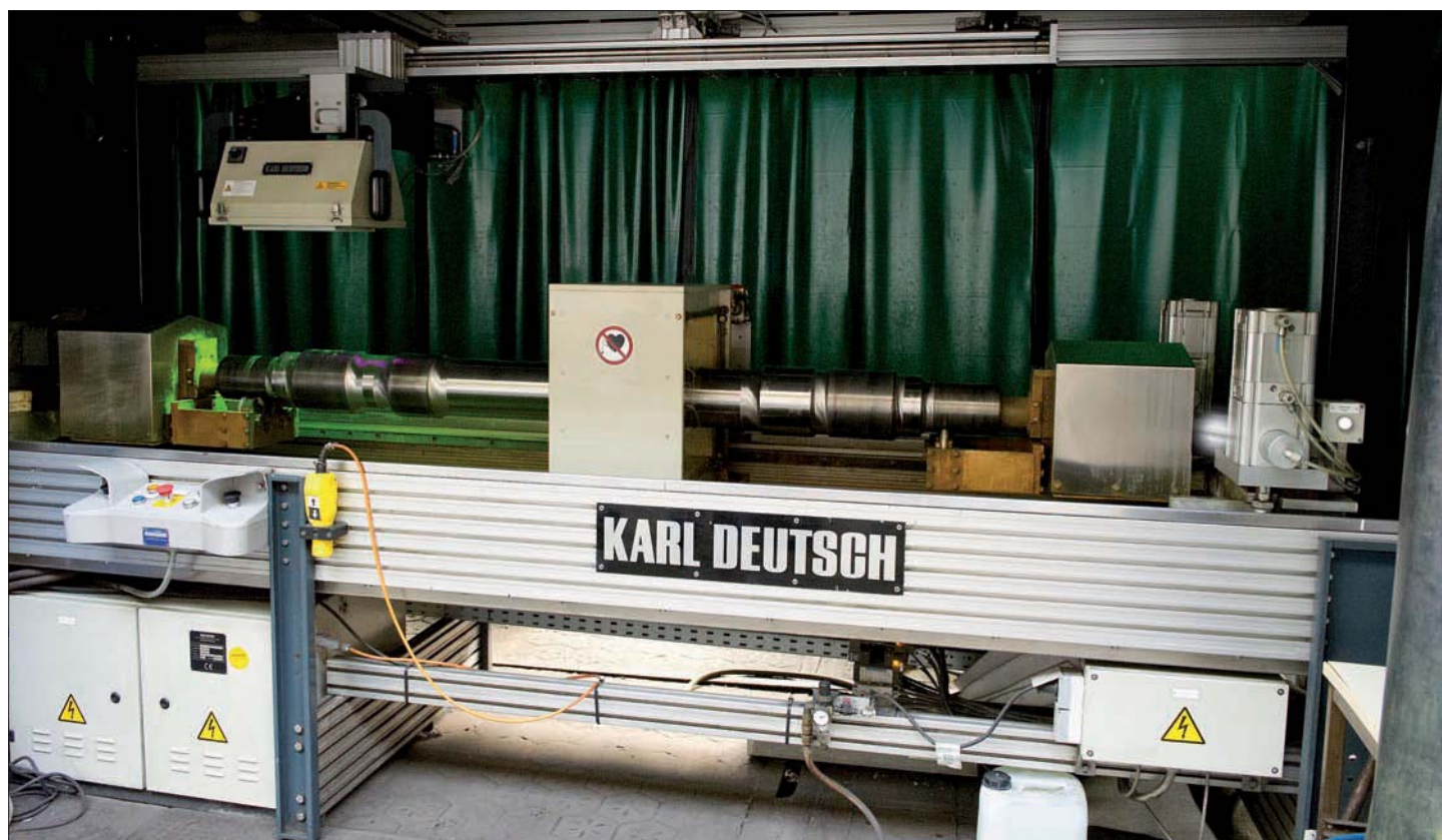
DEUTROFLUX UWS for testing of railway axles: For the inspection of the complete axle shaft a rotating support unit is used. Three UV large area lamps provide uniform illumination. The lamp mounts and the roof of the darkening cabin can be moved pneumatically to enable crane loading from top.
