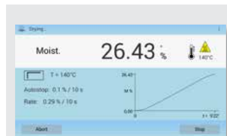
Real-time graph of ongoing drying process
